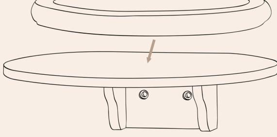
2 dowels and screws are needed to fix the bed on the wall. Please note that these dowels and screws are not included and depends on type of your wall.
